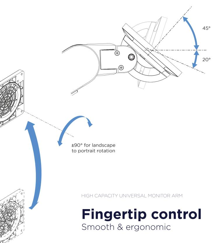
Every joint offers freedom to move, activated with the touch of a finger. Ora 10 comes standard with a rotation limiter and lock.
